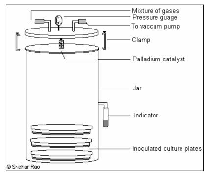
The presence of air is deleterious for many anaerobic bacteria and must be incubated in its absence. The inoculated culture plates are placed inside a metal jar and the lid clamped tight. The air inside is removed using a vacuum pump. The pressure inside the chamber is reduced to 100 mm below mercury.
